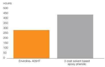
$^{\star}$ The time to clean and blast tank, apply and allow coating to cure and return to service
